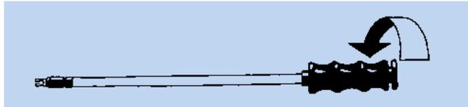
2. Push the introducer so that the distal tip extends out of the sheath and rotate the introducer to lock it in the sheath. (spring compressed)
